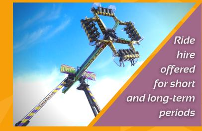
This incredible ride features 16 outward-facing spinning and free looping seats as well as swinging 24 metres over the top in a 360° action, allowing passengers to experience both a weightless sensation and forces of 4.5g - unbelievable dynamics that offer unrivaled thrills!
